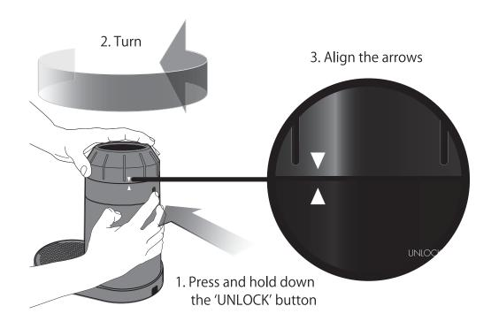
Press and hold down the 'UNLOCK' button at the rear of the motor base and with the other hand turn the grind adjustment collar counterclockwise until the graphic arrow on the collar is aligned with the arrow on the motor base.
