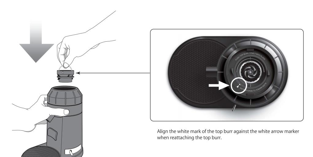
Replace the top burr back into position in the grind adjustment collar and turn clockwise to the desired grind setting.
