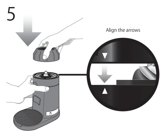
Once both burrs are cleaned, return the grind adjustment collar to its position in the motor base. With the grind adjustment collar in hand, align the arrow on the collar with the arrow on the rear of the motor base and press down.
