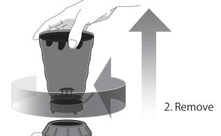
Remove the bean hopper from the motor base, push down and turn counterclockwise. 2
