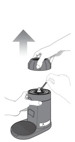
Lift the grind adjustment collar away from the motor base and clean with the brush. Clean the bottom burr using the burr cleaning brush.
